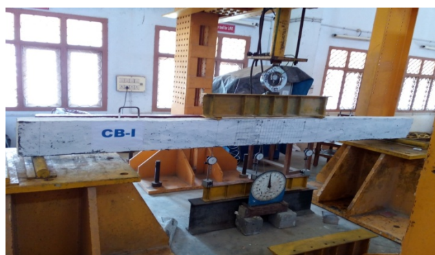
Figure 3 Testing of Beam under Two Point loading
