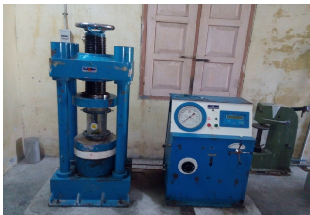
Figure 2 Test Setup for Cylinder Testing
