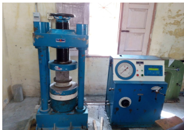
Figure 1 Test Setup for Cube Testing
